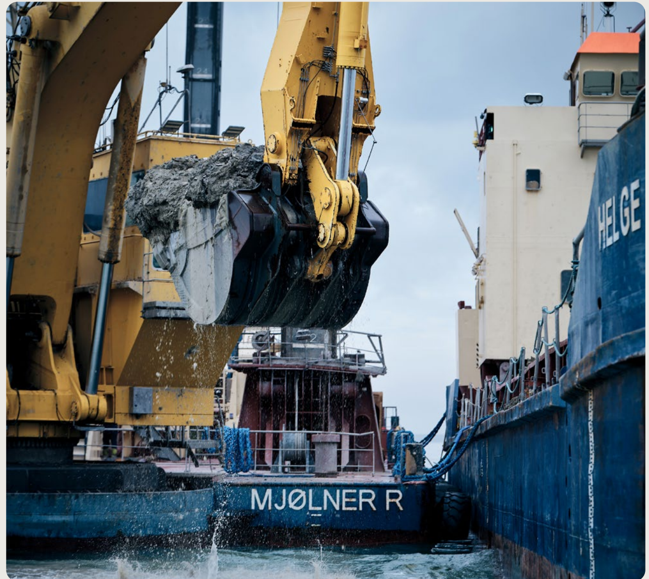
Dredging of clayey material with our backhoe Mjølner R and barge Helge R
